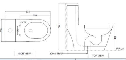
ALL DIMENSIONS ARE IN MM. (TOLERANCE ± 5 MM)
