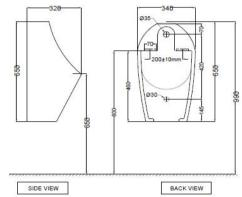
ALL DIMENSIONS ARE IN MM. (TOLERANCE ± 5 MM)
