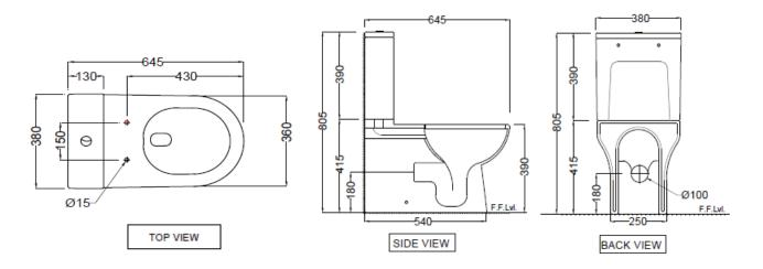
ALL DIMENSIONS ARE IN MM. (TOLERANCE ± 5 MM)
